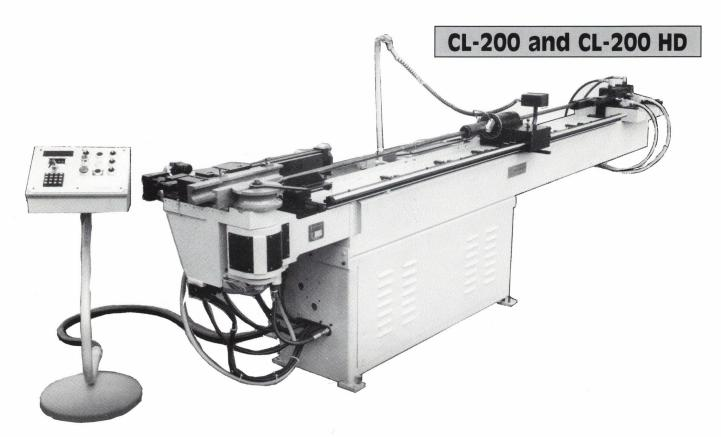
The CL-200 and CL-200 HD benders are noted for reliability and productivity. The clamp and pressure die bolsters mount on hard, precision ground steel slides riding on fitted bronze ways.
